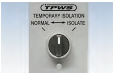
TPWS temporary isolation switch
