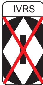
Lineside sign placed at exit from an area where IVRS should be used
