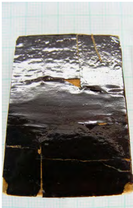
(a) Specimen consolidated with Mowiol 3-83 in the areas towards the rear and the front end of the board.
