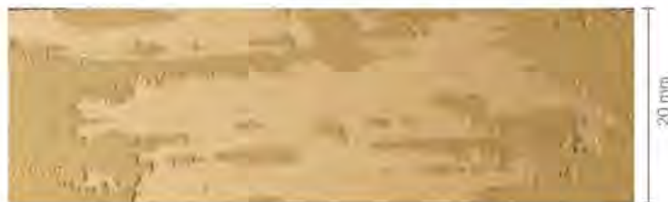
Figure 7.6.: Type A DCB fracture surface (detail), resembling the naturally-induced damage on export-type lacquer coating in Figure 7.7b.
