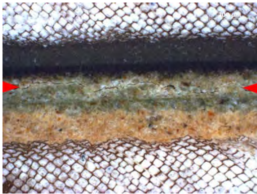
(c) Paraloid B 72 in acetone (type B); showing visible old fracture path and a typical starved bondline, with higher concentration of consolidant away from the bond.
