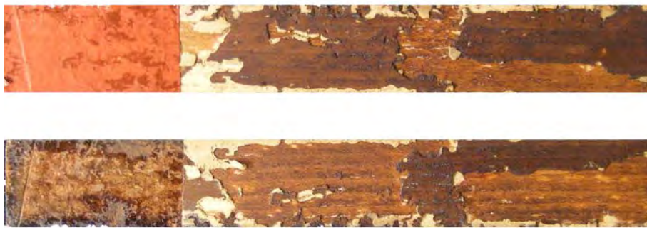
Figure 7.26.: Fracture surfaces of type A DCB specimen consolidated with ki-urushi .
