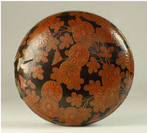
(a) Lid showing blistering and flaking of lacquer coating in the area covering end-grain of the turned wood substrate.
