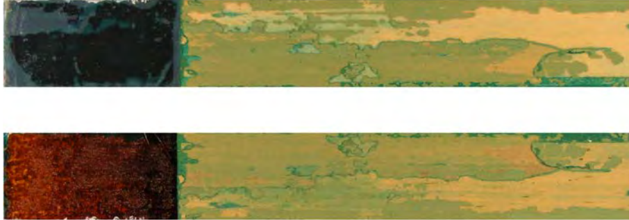
Figure 7.24.: Type B DCB specimen consolidated with starch/isinglass showing typical fracture surfaces with a high proportion of SCF within consolidated and unconsolidated areas of the foundation, as well as some new AF and a negligible degree of failure between the old, consolidated and re-adhered fracture surfaces.
