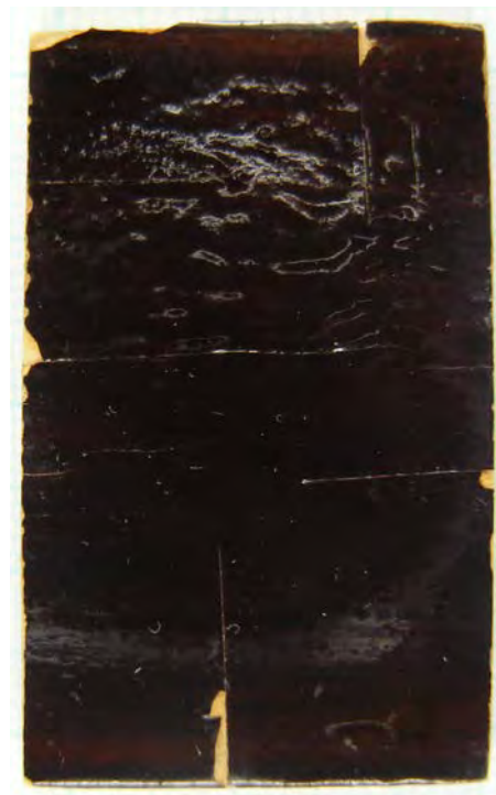
(b) Test specimen consolidated with hide glue in the area of the upper half of the board.
