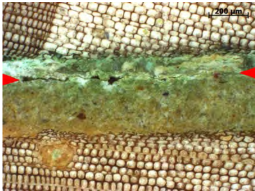
(a) Cold-liquid fish glue (type A); showing good penetration, but leaving voids in the bond along the old fracture surfaces.
