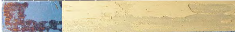
(a) Cohesive failure within the foundation layer and at the wood/foundation interface.
