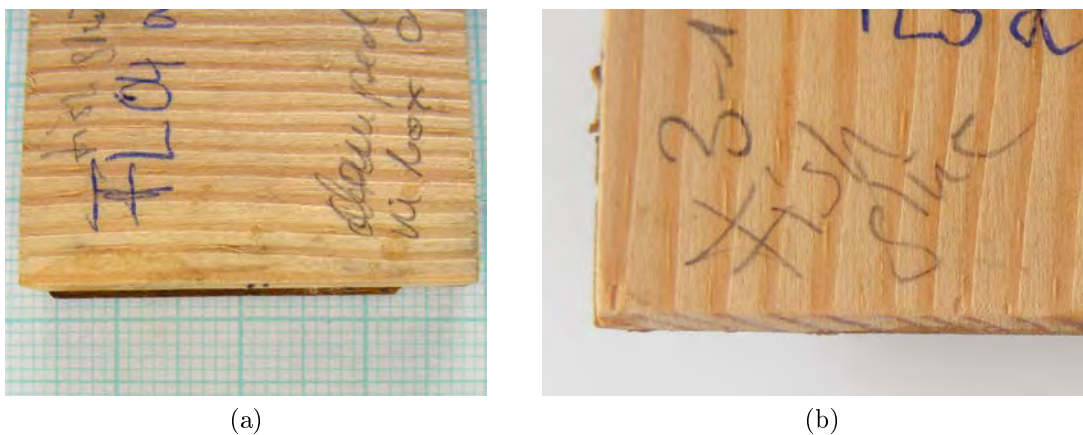
Figure 7.57.: Back side of lifting lacquer specimen board consolidated with Lee Valley fish glue. The formerly lifting coating is protruding over the edge of the substrate (a), whilst the specimen sides along the end-grain show no such coating protrusion (b).
