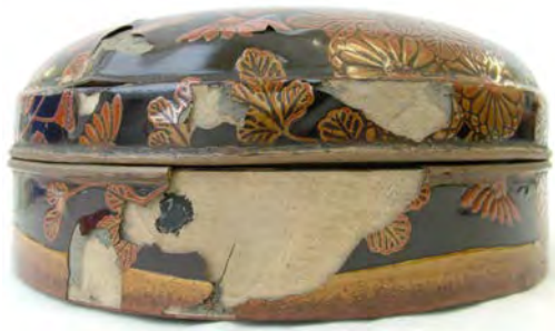
(a) Round box (W.332-1921). Extensive coating losses of the lacquer coating expose the wood substrate. (6.5 x 14.5 cm).
