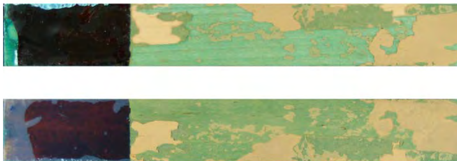
Figure 7.23.: Fracture surfaces of type B DCB specimen consolidated with 10 % bovine hide glue solution stained with Fast Green.
