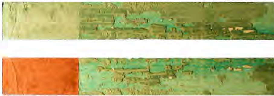
Figure 7.21.: Example of typical fracture surface of DCB specimen type A consolidated with cold-liquid fish glue stained with Fast Green).
