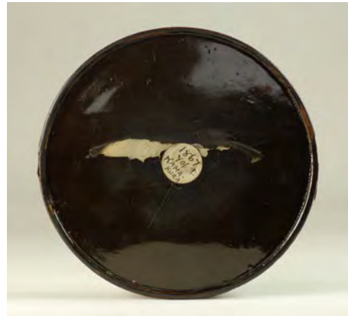
(b) Underside of base, showing a large collapsed blister in the lacquer coating parallel to the grain direction of the wood substrate.
