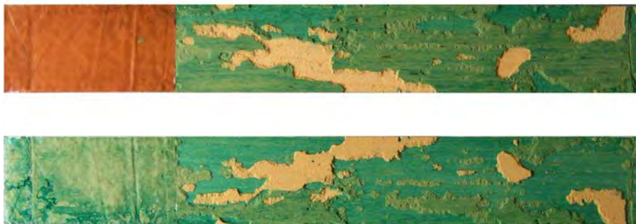
Figure 7.20.: Fracture surfaces of DCB specimen consolidated with 10 % isinglass solution stained with Fast Green.
