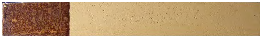
(a) Cohesive failure within the foundation layer and at the wood/foundation interface.
