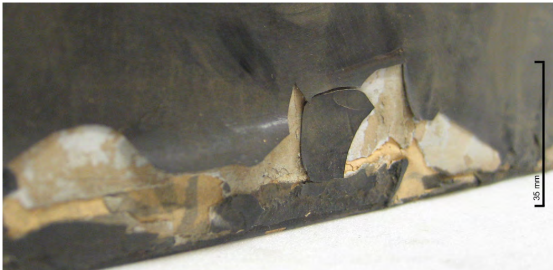
Figure 1.1.: Detail of a Japanese shrine panel (W.1-1913) showing losses in the lacquer coating caused by delamination and lifting of its multilayered coating structure. (Photograph by N. Schellmann, courtesy of the V&A).
