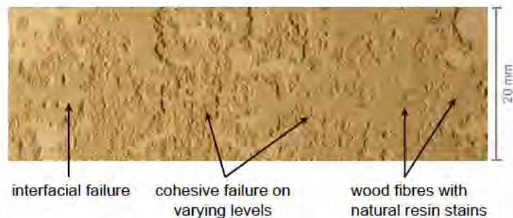
Figure 7.4.: Type A DCB specimen: detail of the fracture surface of a foundation layer located between two wood interfaces before testing, showing failure on varying levels.
