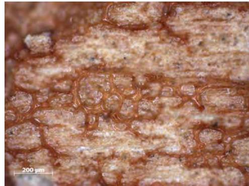
(b) Cohesively failed Mowilith DMC2 layer showing significant plastic deformation (ductile drawing and void coalescence) which caused the bridging observed.
