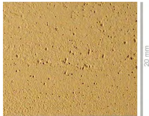
(b) Detail of typical DCB specimen type B with pinholes of varying diameter.
