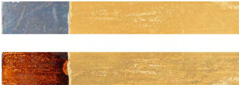
Figure 7.36.: Fracture surfaces of DCB specimens consolidated with Mowiol 3-83 (unstained), showing failure within the bondline between the consolidated and re-adhered old fracture surfaces, and small areas of SCF within unconsolidated parts of the foundation.
