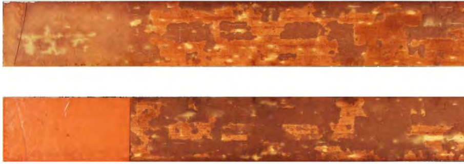
Figure 7.38.: Fracture surface of DCB specimen consolidated with Mowilith 50 (20%) in toluene, stained with Lugol's solution.
