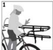
1 Squeeze handle and pull down rack
