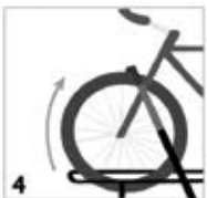
4 Pull on hook to extend and then lift over tire
