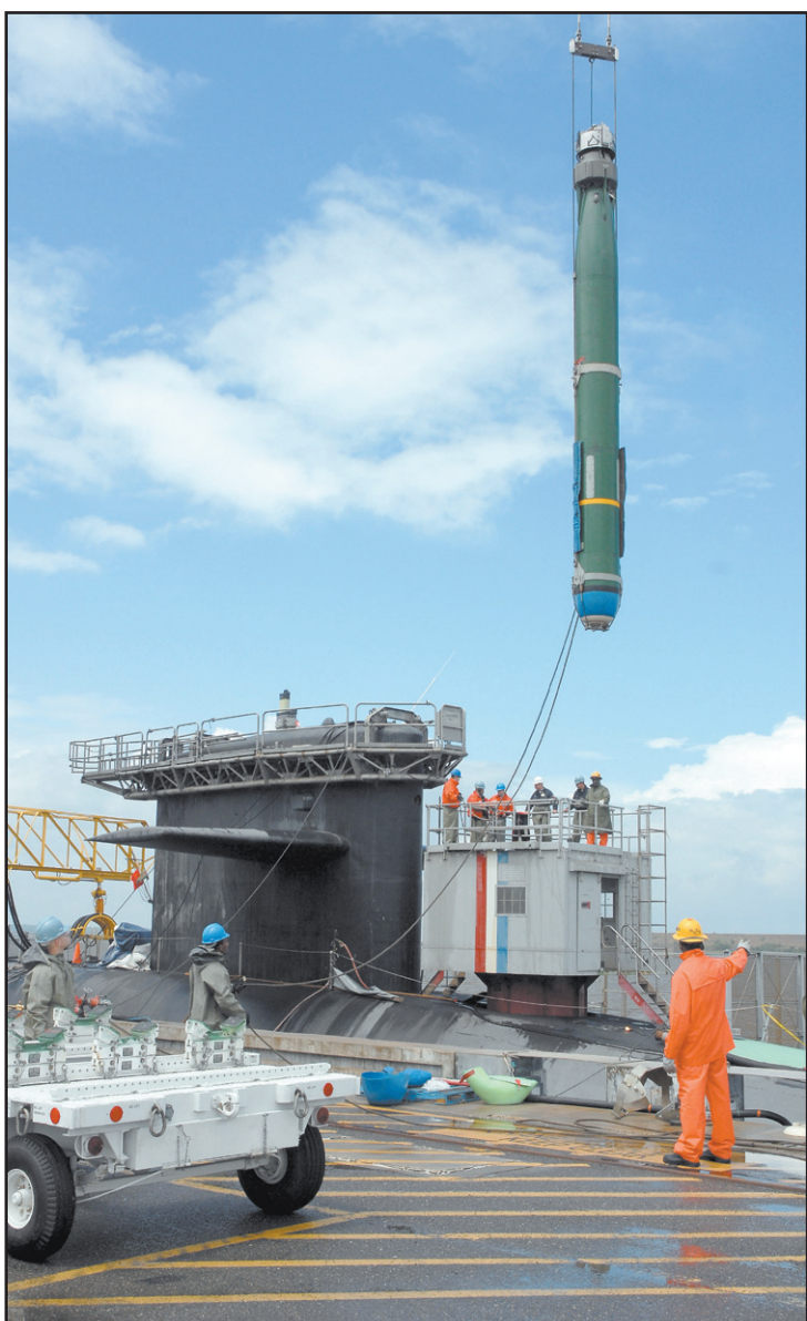
The Defense Ordnance Supply Facility (DOSF) can usually load approximately one dozen torpedoes onto a submarine in one day, depending on weather conditions and the efficiency of the crew receiving the weapons. DOSF receives, prepares and loads several different types of torpedoes, submarine countermeasures, Tomahawk missiles, and emergency beacons onto every submarine operating from Kings Bay.
