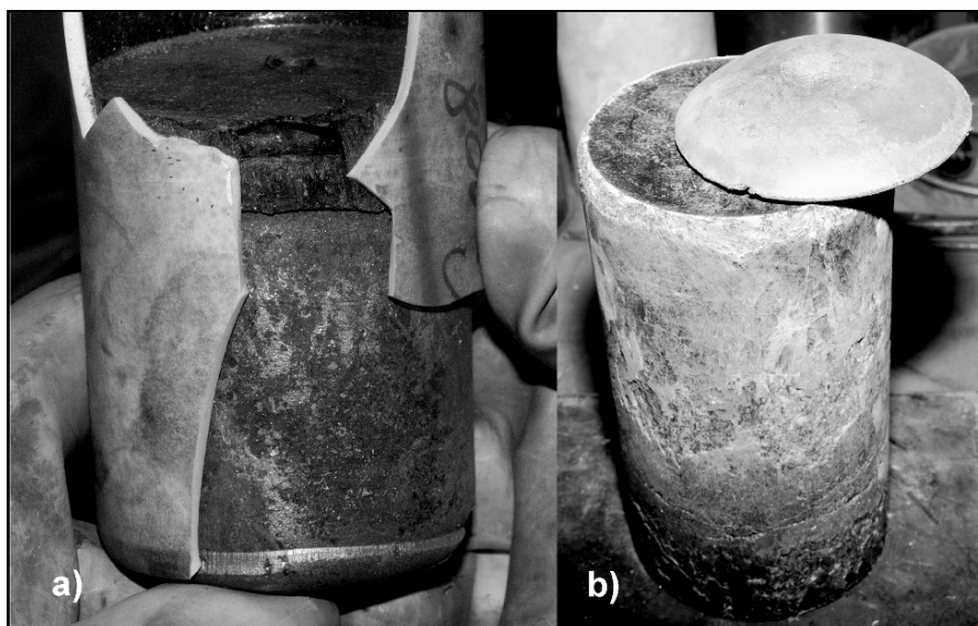
Fig. 7.12 (a) A photograph of a DOR breakout showing the MgO crucible, residues, and metal product at the bottom. (b) The DOR metal button (top) and residues (photographs courtesy of Los Alamos National Laboratory).
