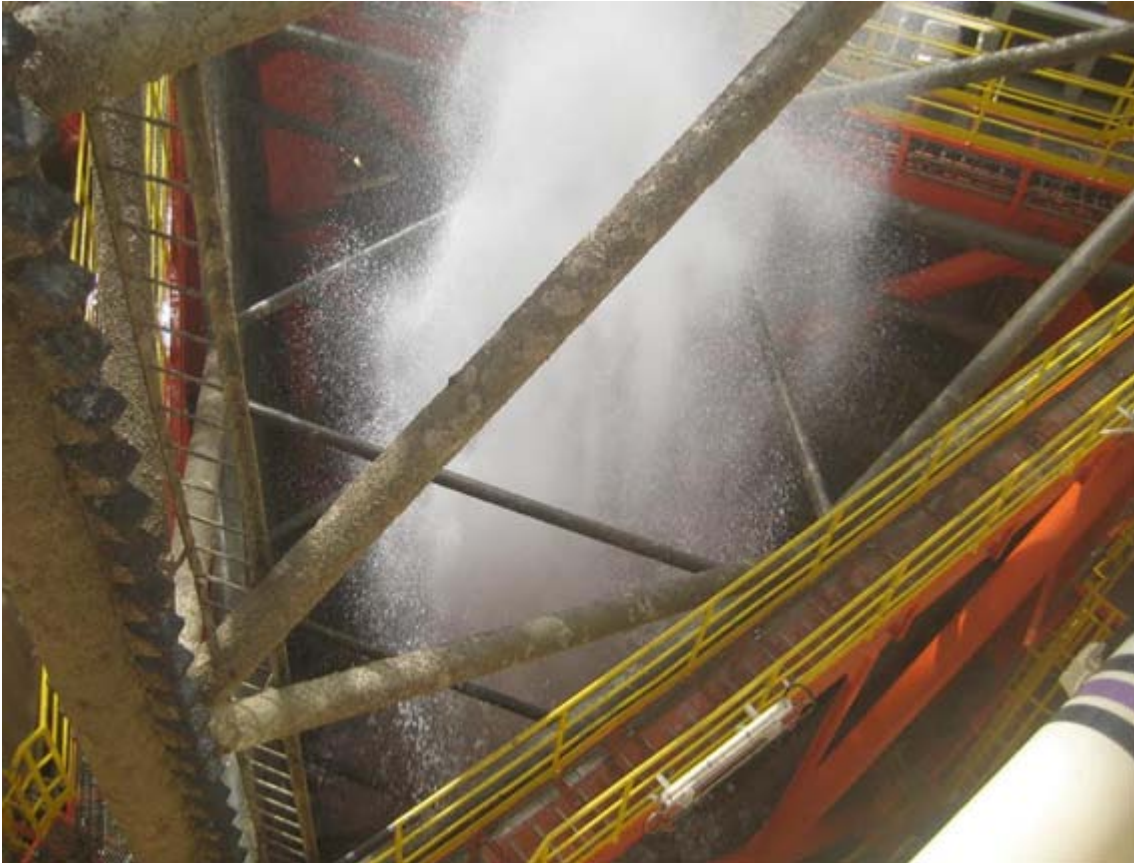
Seen onboard the WEST CASTOR in Brunei while filling up the bow leg empty spud can. The air "trapped" created this nearly 30 m spray. Photo : Richard Qualm - DNV GL – Oil & Gas Thailand ©
