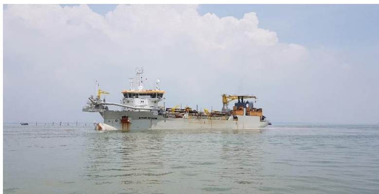
Maintenance dredging works at MICT Access Channel and Basin – TSHD Vitus Bering
