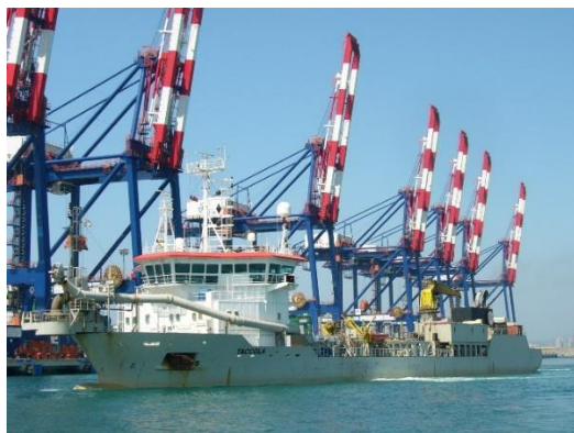
Capital dredging and reclamation works in the port of Taipei – TSHD Taccola (Taiwan)
