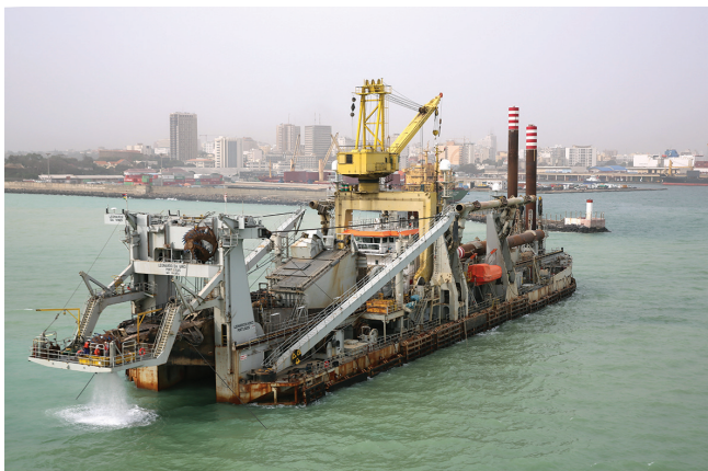
CSD Leonardo da Vinci - Dredging of Access Channel - Dakar (Senegal)
