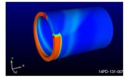
Figure 5. AR Annular RDECFD computation showing fuel behind detonation travelling upstream until propellant total pressure exceeds downstream pressure, upon which typical triangular profile emerges.
