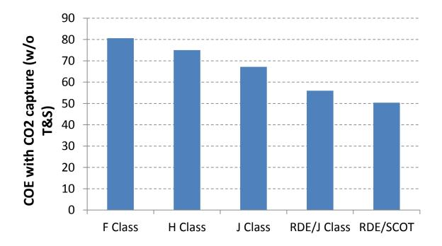
Figure 9. Levelized cost of electricity of various commercial power plants compared with RDE based power plants.
