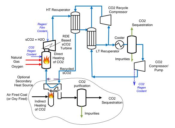
Figure 6. Schematic of a power plant with CO<sub>2</sub> capture incorporating pressure gain combustion in a supercritical CO<sub>2</sub> RCBC which uses natural gas oxy combustion with an optional coal combustion in a boiler with indirectly heating CO<sub>2</sub>.
