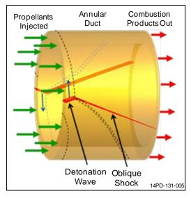
Figure 2. Schematic of a Rotating Detonation Engine
