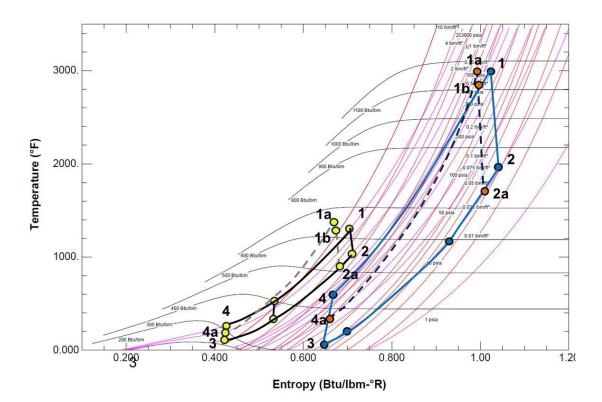
Figure 7. Temperature entropy diagram of a super and sub-critical recompression Brayton
