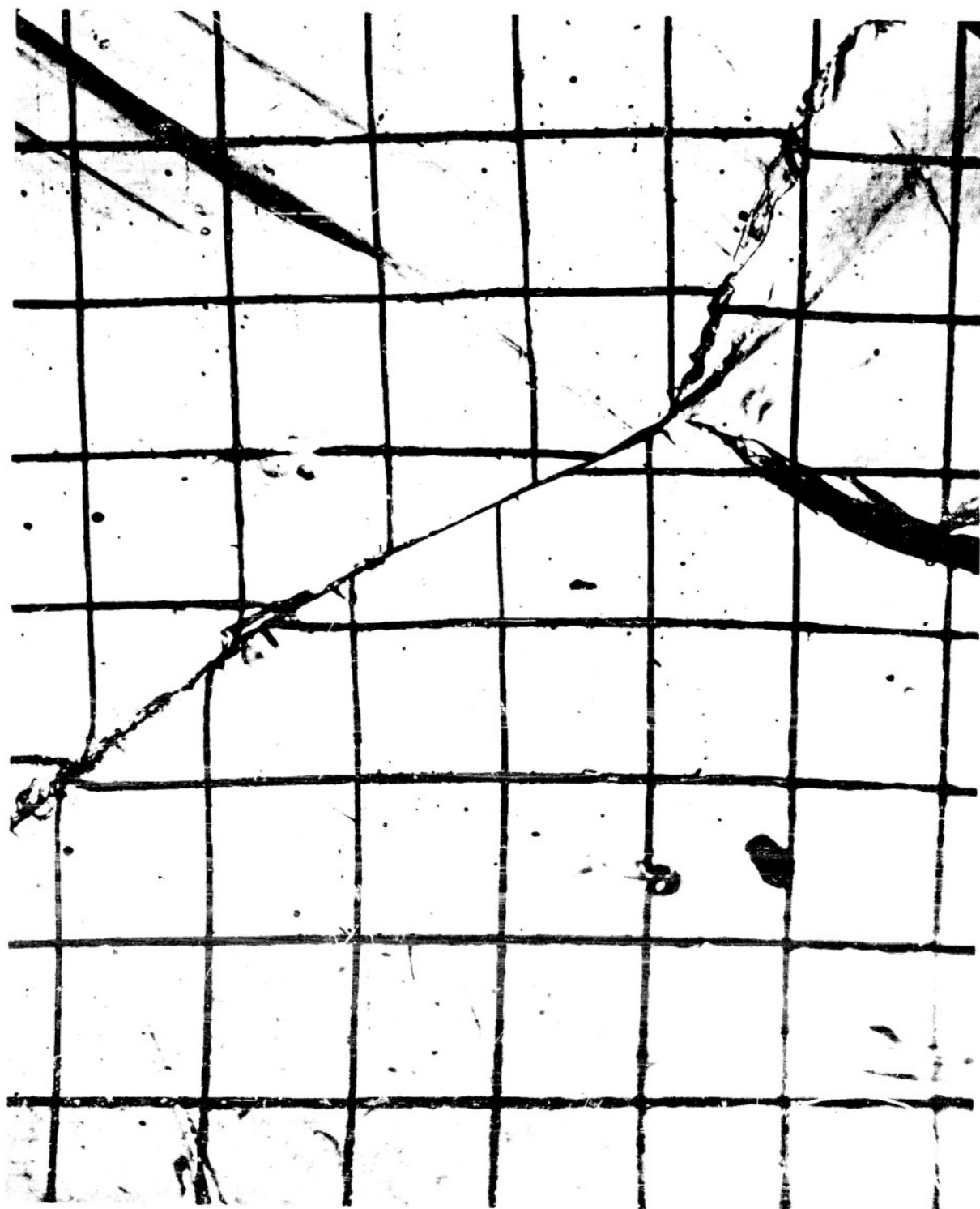
FIG. 1 SHEAR ALONG A GRAIN BOUNDARY IN HIGH PURITY ALUMINUM. CREEP STRESS = 250 PSI, \epsilon_t = 0.07 , T = 610^\circ\text{K} . MAGNIFICATION 100 X.
