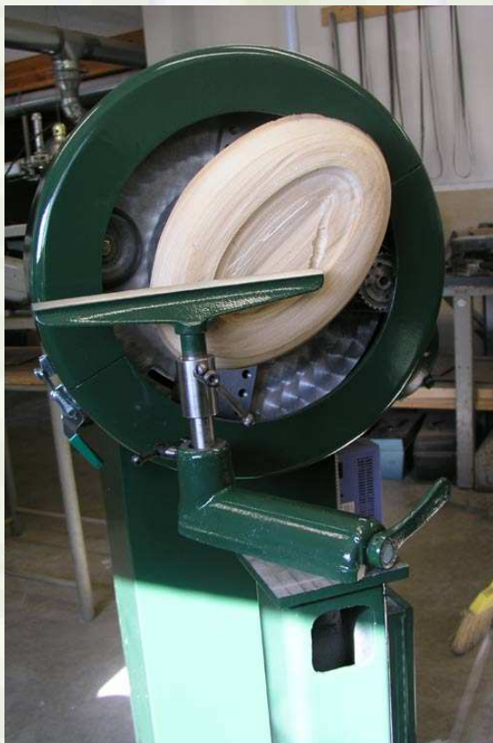
Figure 3405 Bollinger Ovalturning Lathe (BOTULA) [6.3]
