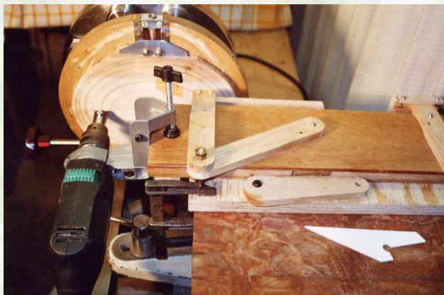
Figure 6307 Routing motor with circle cutter at a straight line linkage (Workshop J. Volmer, Chemnitz 2003)
