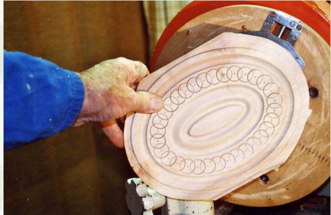
Figure 6306 Lid of a chip box with 32 equally spaced circles forming the Barley-Corn-Pattern (Workshop J. Volmer, Chemnitz 2003)
