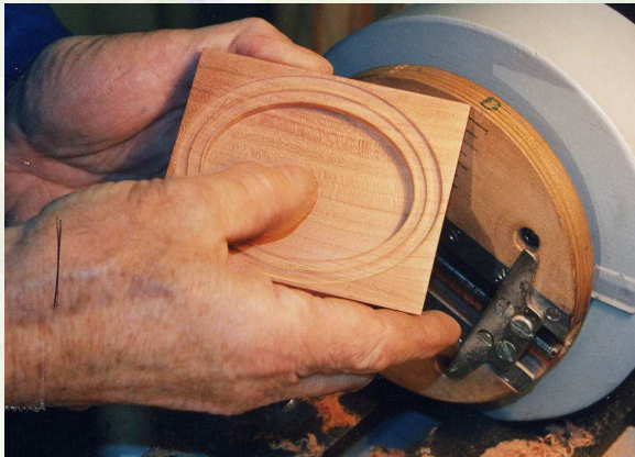
Figure 5408 Sanding the profile near the central line
