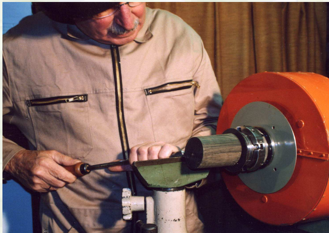
Figure 5601 Box of long grain bog oak in VICMARC Four-Jaw-Chuck on the ODM30
