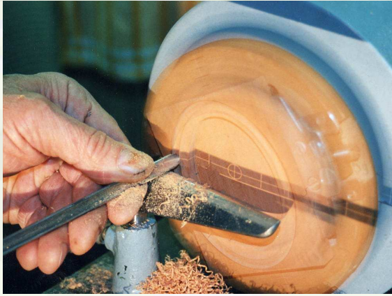
Figure 5407 Turning the profile and the recess
