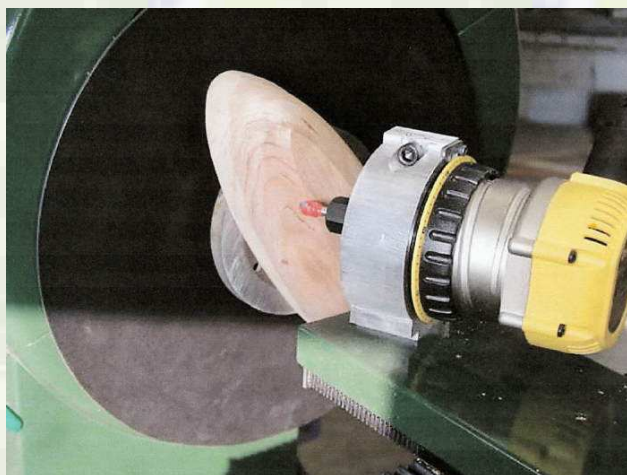
Figure 5206 Routing-Motor with chucked Two-Knife-Ball-Cutter, fixed in a compound slide rest, milling the underside of a bowl at the Bollinger Ovalturning Lathe (BOTULA) [6.3]
