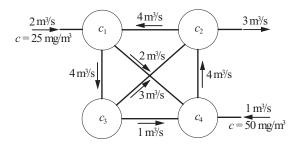
Four mixing tanks are connected by pipes. The fluid in the system is pumped through the pipes at the rates shown in the figure. The fluid entering the system contains a chemical of concentration c as indicated. Determine the concentration of the chemical in the four tanks, assuming a steady state.
