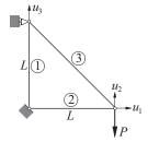
The displacement formulation of the truss shown results in the following simultaneous equations for the joint displacements  $\mathbf{u}$ :
