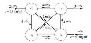
Four mixing tanks are connected by pipes. The fluid in the system is pumped through the pipes at the rates shown in the figure. The fluid entering the system contains a chemical of concentration c as indicated. The rate at which the mass of the chemical changes in tank i is
