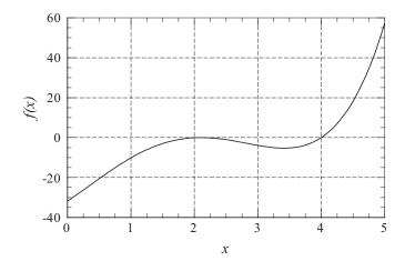
**Solution.** Inspecting the plot of the function, we suspect that the smallest positive zero is a double root at about x=2. Bisection and Ridder's method would not work here, because they depend on the function changing its sign at the root. The same argument applies to the function newtonRaphson. Yet there is no reason why the unrefined version of the Newton-Raphson method should not succeed. We used the following program, which prints the number of iterations in addition to the root:
