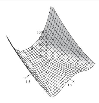
with Powell's method starting at the point (-1, 1). This function has an interesting topology. The minimum value of F occurs at the point (1, 1), But there is a considerable hump between the starting and minimum points that the algorithm must negotiate.
