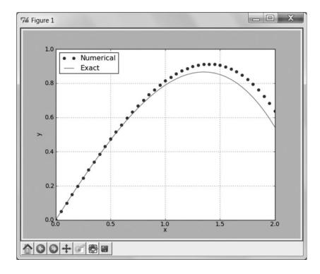
The initial portion of the plot is almost a straight line. Because the truncation error in the numerical solution is proportional to y'', the discrepancy between the two solutions is small. As the curvature of the plot increases, so does the truncation error.
