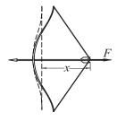
The following table gives the pull F of the bow as a function of the draw x. If the bow is drawn 0.5 m, determine the speed of the 0.075-kg arrow when it leaves the bow. *Hint*: The kinetic energy of the arrow equals the work done in drawing the bow; that is,  $mv^2/2 = \int_0^{0.5 \text{m}} F \, dx$ .
