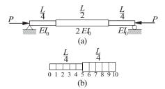
The simply supported column in Figure (a) consists of three segments with the bending rigidities shown. If only the first buckling mode is of interest, it is sufficient to model half of the beam as shown in Figure (b). The differential equation for the lateral displacement u(x) is
