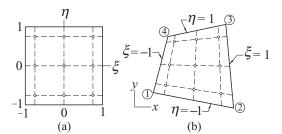
**Figure 6.7.** Mapping of quadrilateral into a rectangle.
