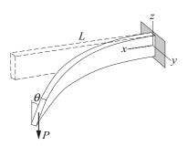
When the depth/width ratio of a beam is large, lateral buckling may occur. The differential equation that governs lateral buckling of the cantilever beam shown is
