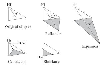
Figure 10.4. Allowed moves of a simplex.
