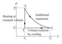
The figure shows the thermodynamic cycle of an engine. The efficiency of this engine for monatomic gas is
