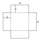
The sheet of cardboard is folded along the dashed lines to form a box with an open top. If the volume of the box is to be 1.0 m<sup>3</sup>, determine the dimensions a and b that would use the least amount of cardboard. Verify the result analytically.
