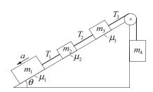
The four blocks of different masses  $m_i$  are connected by ropes of negligible mass. Three of the blocks lie on a inclined plane, the coefficients of friction between the blocks and the plane being  $\mu_i$ . The equations of motion for the blocks can be shown to be
