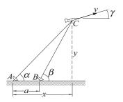
The radar stations A and B, separated by the distance a=500 m, track the plane C by recording the angles  $\alpha$  and  $\beta$  at one-second intervals. If three successive readings are
