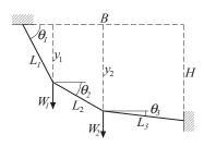
A cable supported at the ends carries the weights  $W_1$  and  $W_2$ . The potential energy of the system is
