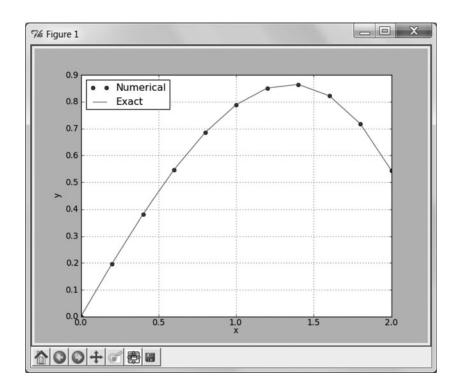
Comparing this plot with that in Example 7.2, we see the clear superiority of the fourth-order Runge-Kutta method over Euler's method. In this problem, the two methods involve about the same amount of computation. Euler's method requires one evaluation of  $\mathbf{F}(x, \mathbf{y})$  per step, whereas the Runge-Kutta method involves four evaluations. Yet Euler's method has four times as many steps. Considering the large
