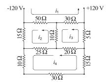
Determine the loop currents  $i_1$  to  $i_4$  in the electrical network shown.
