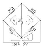
The electrical network shown can be viewed as consisting of three loops. Applying Kirchoff's law ( $\sum$ voltage drops =  $\sum$ voltage sources) to each loop yields the following equations for the loop currents  $i_1$ ,  $i_2$  and  $i_3$ :
