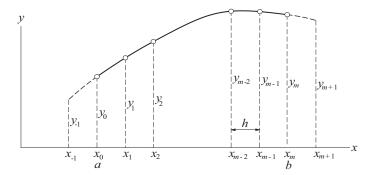
Figure 8.1. Finite difference mesh.
