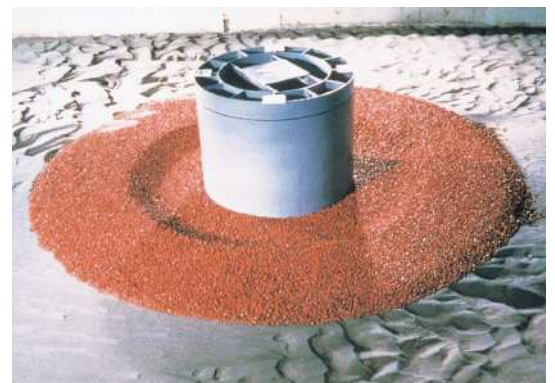
Result of hydraulic model test (with scour protection)
