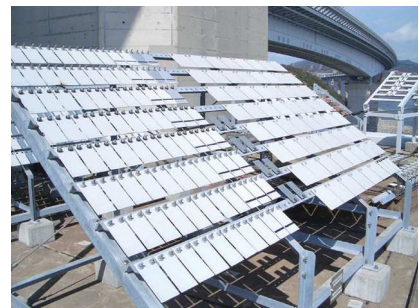
Exposure test for painting
