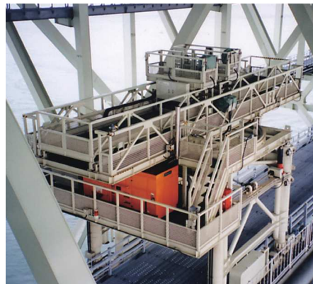
Maintenance vehicle for inside girder (Akashi-Kaikyo Bridge)
