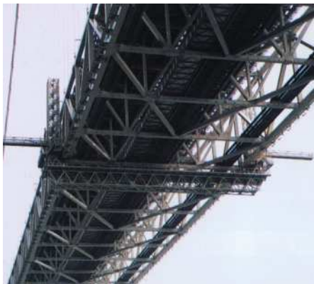
Maintenance vehicle for outside girder (Akashi-Kaikyo Bridge)
