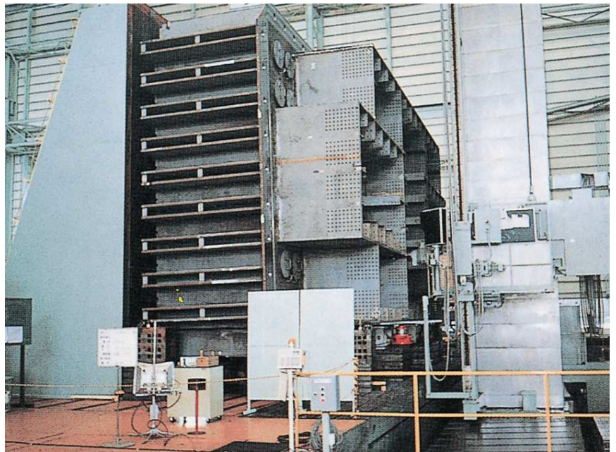
Polishing cross-section of tower shaft using large scale facing machine To control the inclination of the towers and to assure the metal touch at connections, each end of the tower shaft blocks was polished up to 0.0125 mm ruggedness.
