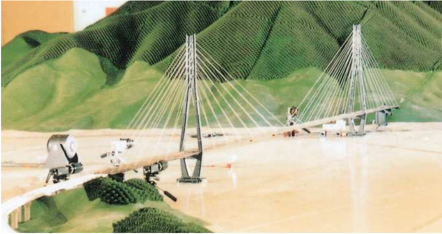
Full-model wind tunnel test to evaluate the influence of topography (Tataro Bridge, scale=1/200)
