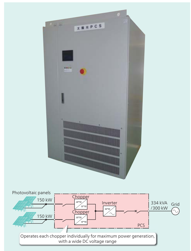
6 300-kW photovoltaic PCS (top) and photovoltaic PCS circuit diagram (bottom)
