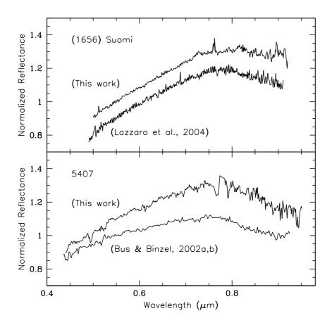
Figure 4: Spectra of asteroid (1656) Suomi (top panel) and 5407 (bottom panel) compared with those obtained by Lazzaro et al. (2004) and Bus and Binzel (2002a,b), respectively. Spectra are normalized to unity at 0.55  $\mu$ m, and are offset for clarity.
