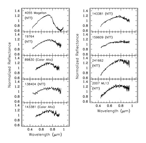
Figure 3: Spectra of NEAs obtained with the NTT and the 2.2 m telescope. The numerical designation for each asteroid is given. All spectra are normalized to unity at 0.55  $\mu$ m. Asteroid 143381 (2003 BC21) was observed with both telescopes, due to bad weather conditions the spectrum obtained with the 2.2 m telescope at Calar Alto looks noisier than the one obtained with the NTT.
