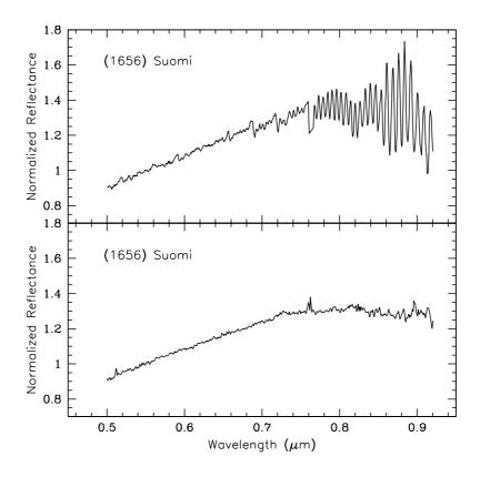
Figure 1: The spectrum of asteroid (1656) Suomi obtained with the 2.2 m telescope using two different detectors, the Lor#11i (top panel) and the SITe-1d (bottom panel). The spectrum obtained with the Lor#11i CCD exhibits strong fringing longwards of 0.7  $\mu$ m. In the present work we only report the data obtained with the SITe-1d CCD.
