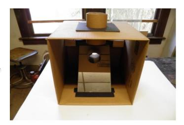
Insert the cardboard tube into the lens barrel collar with the lens facing closest to the mirror.
