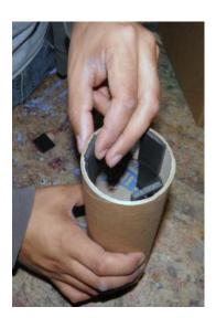
Hot glue three more pieces of cardboard to the tube to keep the lens securely in place.
