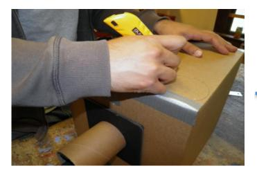
Use the cardboard tube to trace two circles onto the side of the box as shown, opposite the mirror and in the corners closest to the lens barrel.
