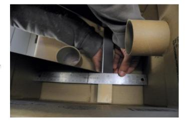
Mounting the mirror can get a little complicated. It is important to mount the mirror inside the box at a 45 degree angle. Use a protractor or 45 degree square to help.
