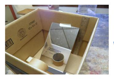
The mounted mirror should have one end on the bottom of the box and the other end attached opposite the lens barrel as pictured.
