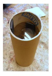
Hot glue 3 small pieces of cardboard 1.5" from one end of the tube. Place the lens inside the tube so it rests on the cardboard pieces.
