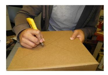
Cut out the lens barrel hole on the box using a utility knife.
