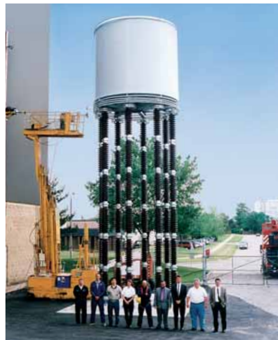
Fig. 5.3-2: Air-insulated smoothing reactor – Tian Guang project
