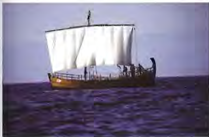
The replica, Kyrenia II, on a voyage between Cyprus and Athens. Her single broad square sail, typical of those seen in ancient vase painting and relief sculpture, was raised upwards like a Venetian blind by the vertical lines seen here. The lines ran through rings sewn to the sail. Over 150 such lead rings were found in the excavation.
