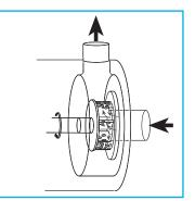
Centrifugal force drives the materials to the periphery of the workhead where they are subjected to a milling action in the gap between the rotor and the stator wall. Agglomerates in the milk powder are broken down as the powder is finely dispersed into the milk.
