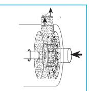
The product is forced out through the stator as fresh materials enter the workhead. In a short mixing cycle all the material passes through the workhead, progressively reducing sugar granule size and exposing an increasing surface area to the milk, accelerating the dissolving process.
