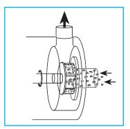
The high speed rotation of the rotor blades creates a powerful suction which draws the milk and sugar granules/milk powder from the vessel into the workhead.
