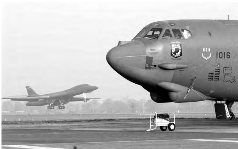
Heavy players. A venerable USAF B-52H bomber stands parked on the ramp at RAF Fairford, England, as a successor-generation B-1B takes off on a mission to deliver as many as 80 500-lb Mk 82 bombs or 30 CBU-87 cluster bomb units against enemy barracks and other area targets. An AGM-86C CALCM fired from standoff range by a B-52 was the first allied weapon to be launched in the war.
