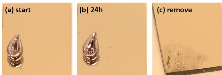
Figure 25 Nb-C film photographed at (a) start of the experiment, (b) 24 hours later and (c) after removal.
