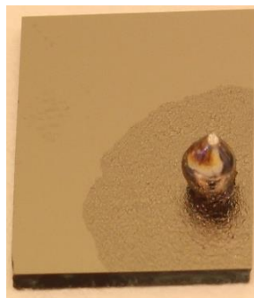
Figure 8 Cr-C rich film with a Galinstan drop. Color-changes of the drop was seen as well as that cracks started to form.
