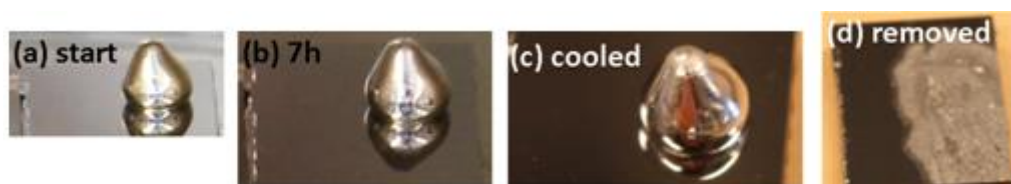
Figure 22 Ti-C film in elevated temperatures at (a) start, (b) 7 hours after application, (c) 5 minutes after the film was pulled out from the furnace and (d) after removal.
