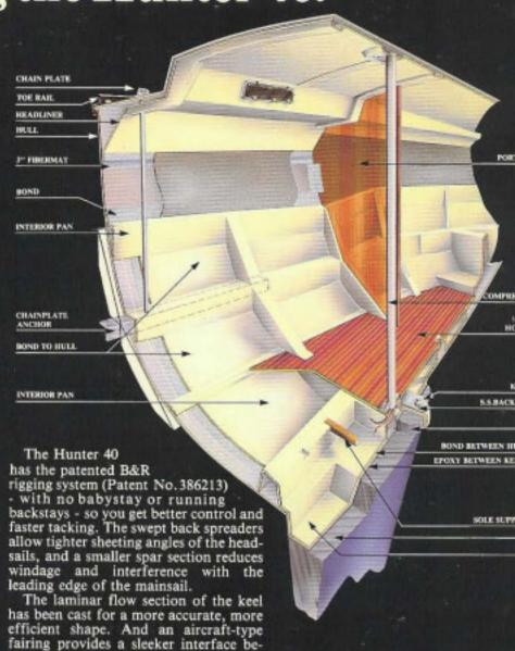
fairing provides a sleeker interface between the hull and the keel. Both the shoal and deep draft keels have sumps and recessed ears that distributes the load between the hull and internal
