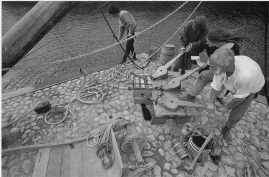
Bellows technology proved more than capable of supplying the diver at moderate depth. Photo: D Lazenby
