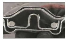
Many rescue tool manufacturers' display their cutters shearing through strengthening bars and HSLA channel with Boron steel bar inserts. Be aware of the cross sectional area in respect of the cut. Where the channel is small it will butt up against the stock where the tool has the most cutting force. This display of the cutters ability is not a true indication of what is actually required.
