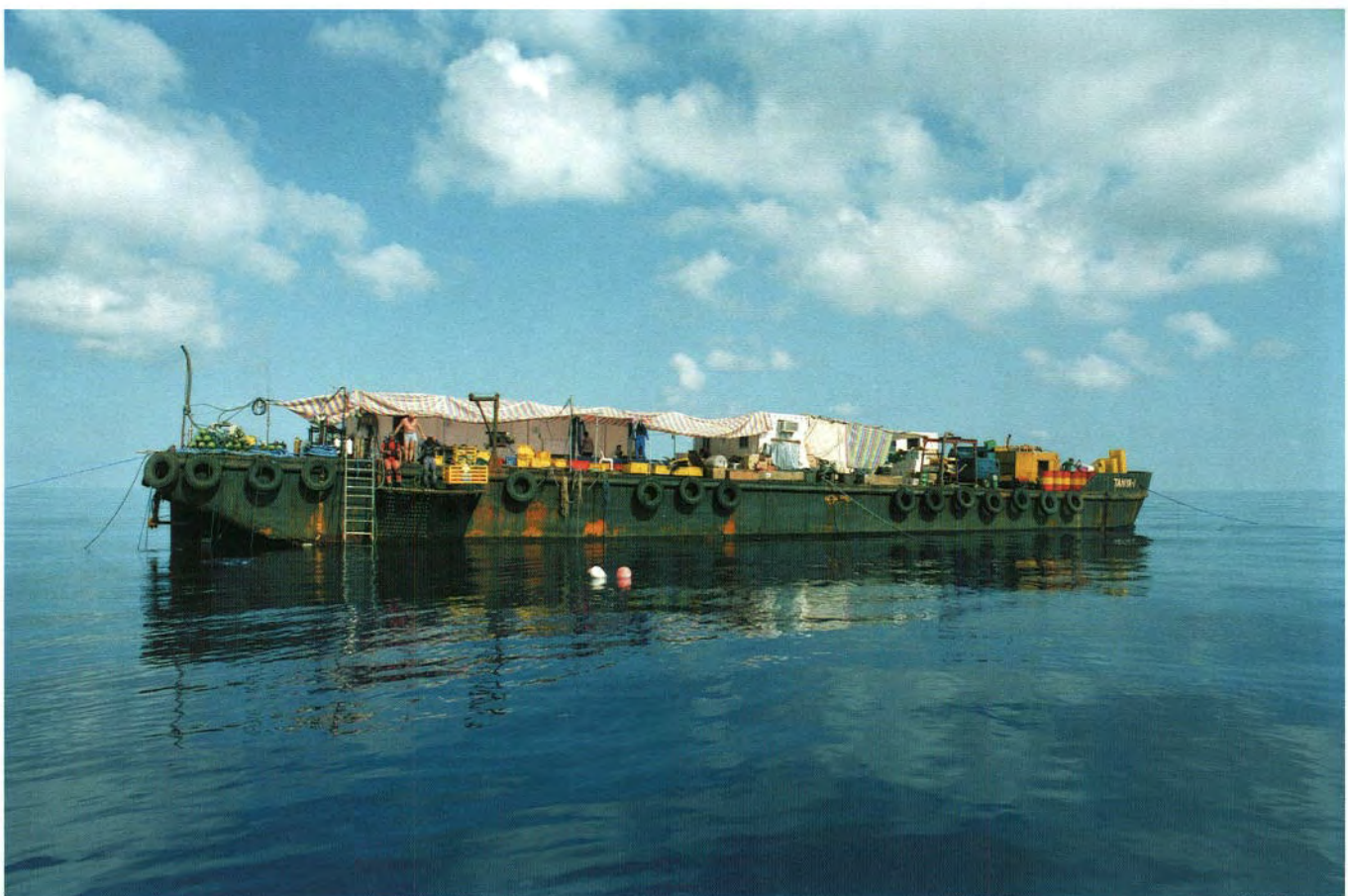
Photo 2. The barge Thania anchored by six anchors over the site.
