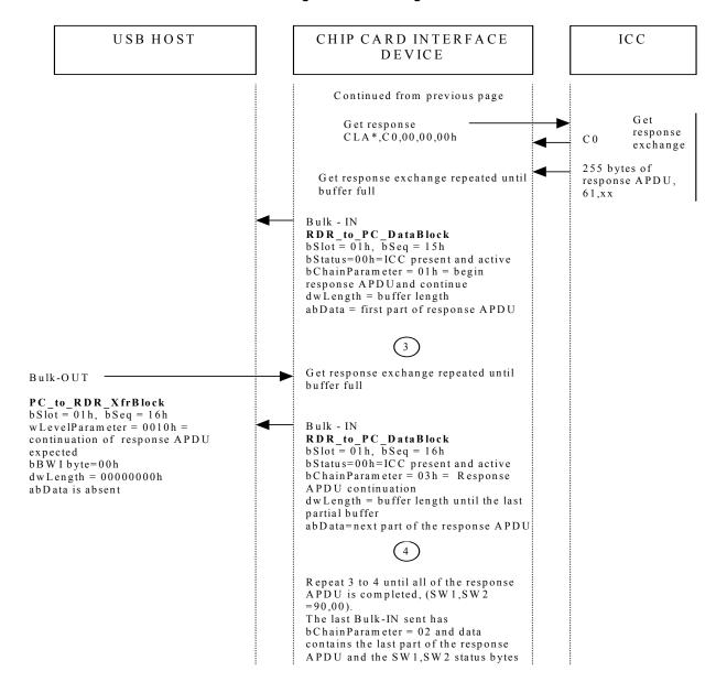
\* The CLA (class) byte for the Get Response command can be one of several values. When an ICC is newly inserted into a slot, the CCID will use the value of the bClassGetResponse field of the Class Descriptor until a PC\_to\_RDR\_T0APDU command message is received which changes the bClassGetResponse value for that slot.
