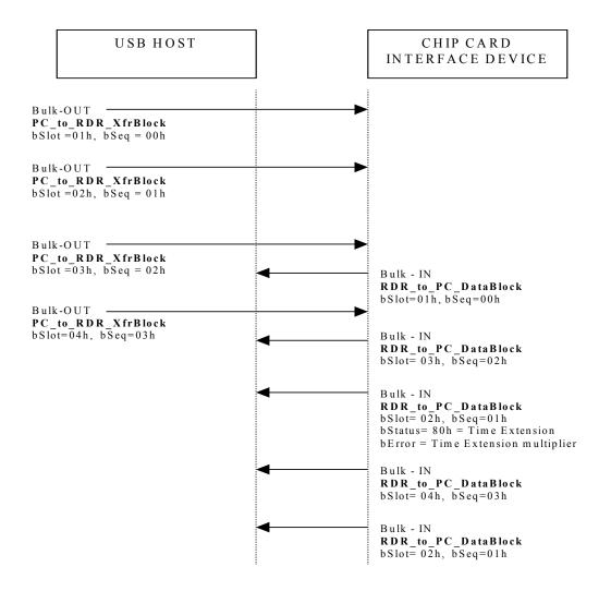
Note: Because the CCID reported bMaxCCIDBusySlots equals 3 – at any time, only 3 active commands are allowable. Responses for different slot commands can be send by the CCID asynchronously upon command completion. The Host keeps information about the active commands and reset it after getting a response. If status byte of a response has Time Extension bit set, the Host will not decrease number of active commands and just wait for a new response with the same bSeq number.
