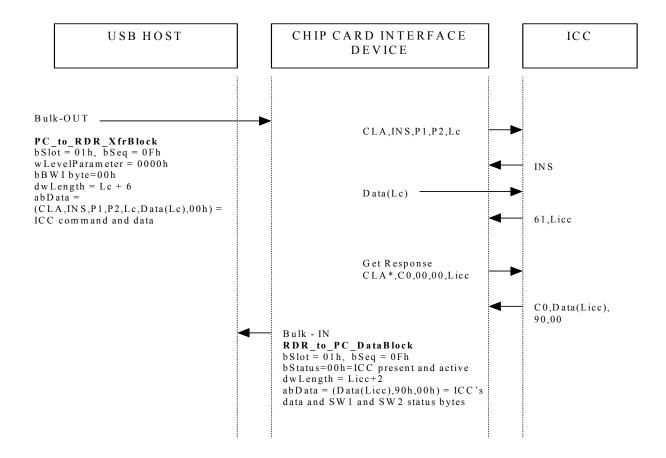
\* The CLA (class) byte for the Get Response command can be one of several values. When an ICC is newly inserted into a slot, the CCID will use the value of the bClassGetResponse field of the Class Descriptor until a PC\_to\_RDR\_T0APDU command message is received which changes the bClassGetResponse value for that slot.
