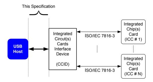
Figure 2-1 Scope of the CCID specification
