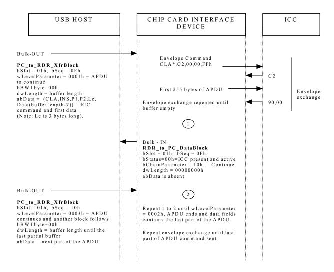
\* The CLA (class) byte for the Envelope command can be one of several values. When an ICC is newly inserted into a slot, the CCID will use the value of the bClassEnvelope field of the Class Descriptor until a PC\_to\_RDR\_T0APDU command message is received which changes the bClassEnvelope value for that slot.
