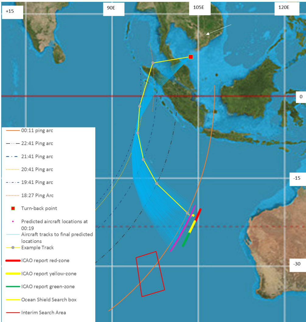
Figure 16: Example fitted track with 18:29UT ping position moved North by adjustment of early speeds, without affecting the BFO values at 20:41UT and later. Also shown are the best fit tracks determined earlier in the paper
