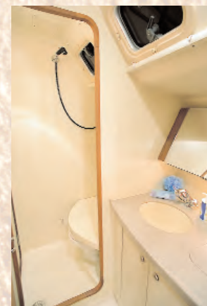
An aft head with integral shower is positioned for convenient access from the aft stateroom or from the salon.
