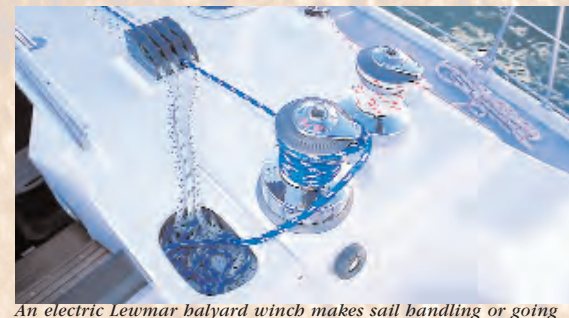
An electric Lewmar balyard winch makes sail banding or going
