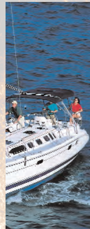
The Hunter trademark cockpit arch keeps the adjustable traveler up and out of the way and makes a great attachment point
