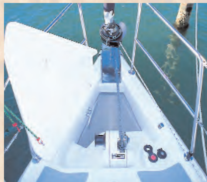
The standard recessed windlass allows the capability of handling two anchors simultaneously on the dual offset anchor roller.
