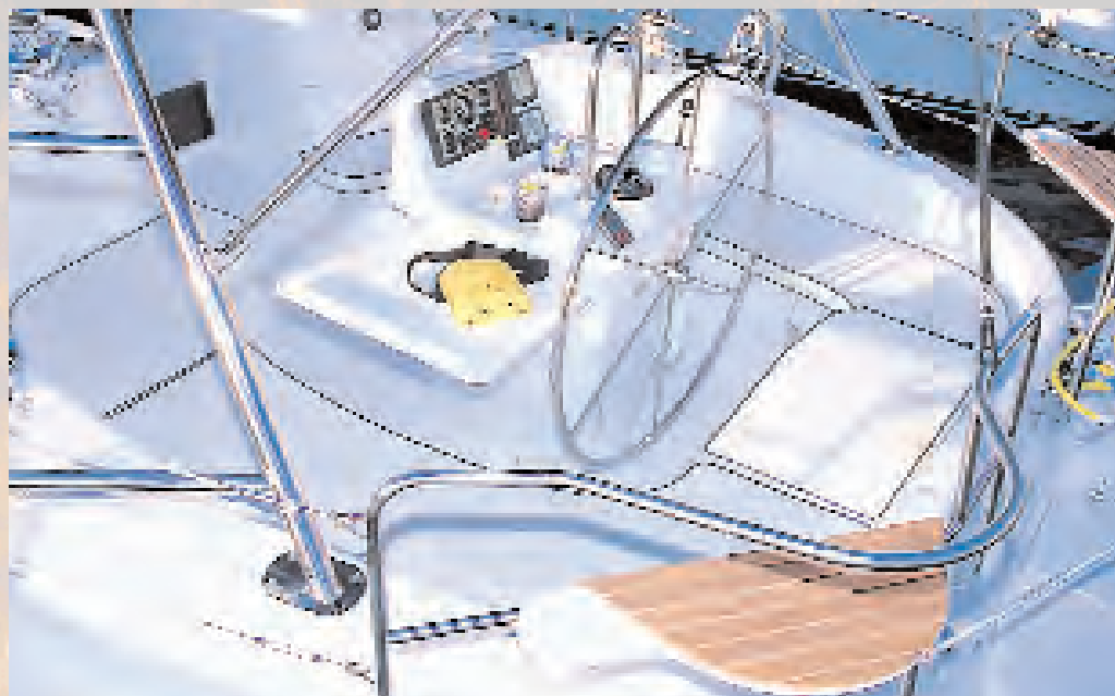
By bringing the cockpit full beam, it allows the use of a custom console complete with mechanical steering, electronics space, twin fold-down tables and even a storage bin with drinkholders.
