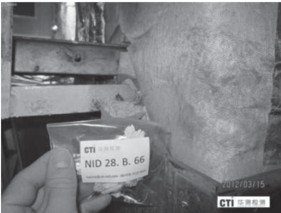
Picture: Insulation material detected containing asbestos from newbuilding ship
