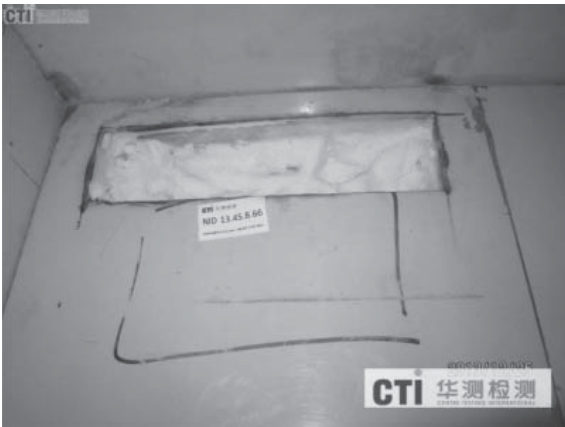
Picture: Cooling chambers material found containing over concentration of ODS as required
