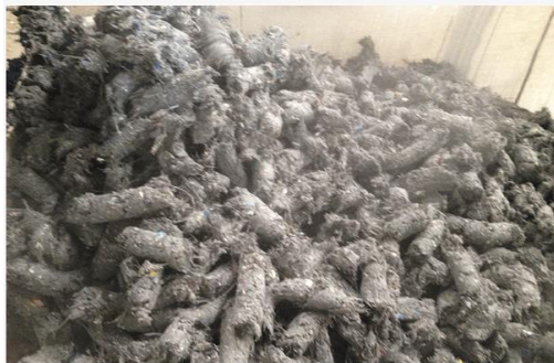
Figure 7. Pellets as the final product from the URENCO waste treatment plant in Hanoi (13).
