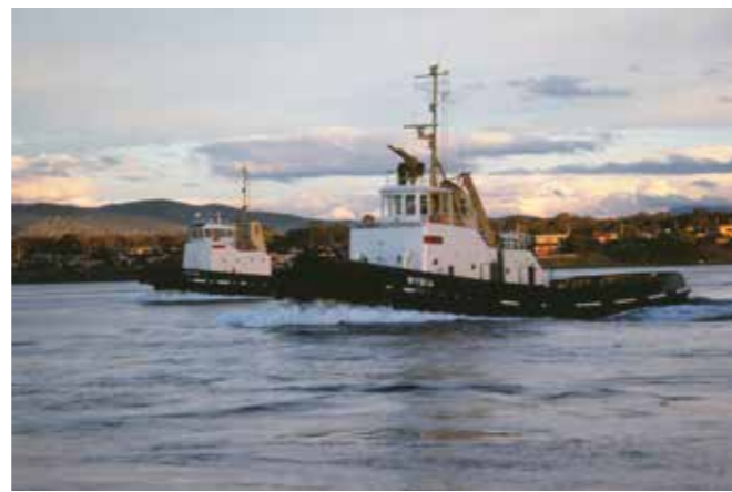
Wybia (2) and Yorktown in Launceston in December 1976. Wybia (2) was Launceston's principal ship-handling tug from 1967, and had a bollard pull (or towing power) of 20 tons—nearly three times that of its predecessor. Photo: K Barr
