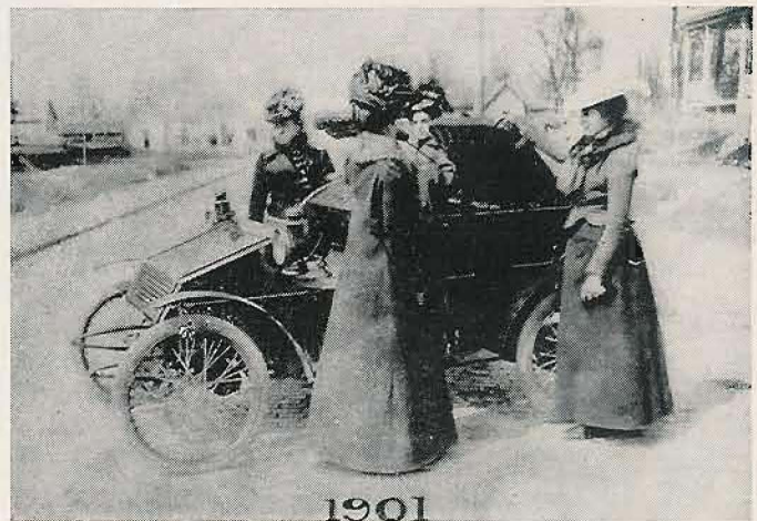
A 1901 experimental model of the car that later became known as the Union, designed and built by John W. Lambert in Union City, Indiana. Note the back seat folded flat providing luggage and equipment space, predating the present drop down station wagon seats.
