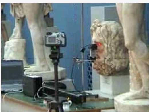
Fig. 6: The iris of the head of Zeus in the Copenhagen Ny Carlsberg Glyptotek is being examined with light from a fiber. The practical value of the probe is that it is easy to get the laser light to the sample, collect the Raman scattered light and send it to the spectrometer, as shown in Fig. 5.
