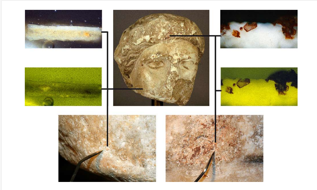
Fig. 2: IN 2830. Paint samples 1+2, top center: head with location of samples (bottom left and right are details); top and centre left: Sample 1 (flesh colour) in tungsten light and UV-FL; top and centre right: Sample 2 (damaged area at forehead and hairline) in tungsten light and UV-FL.
