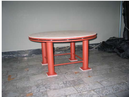
Fig. 4: Heavy duty steel turntable with degree markings. Height 50 cm. Museum photo.
