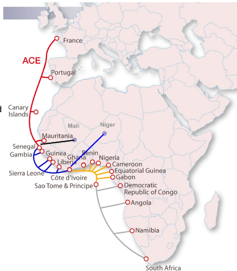
Figure 30: Current Configuration of ACE submarine Cable stations
