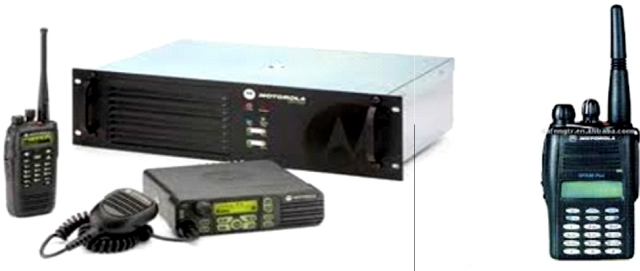
Figure 27: Private Mobile Radio (PMR) base station and handsets
