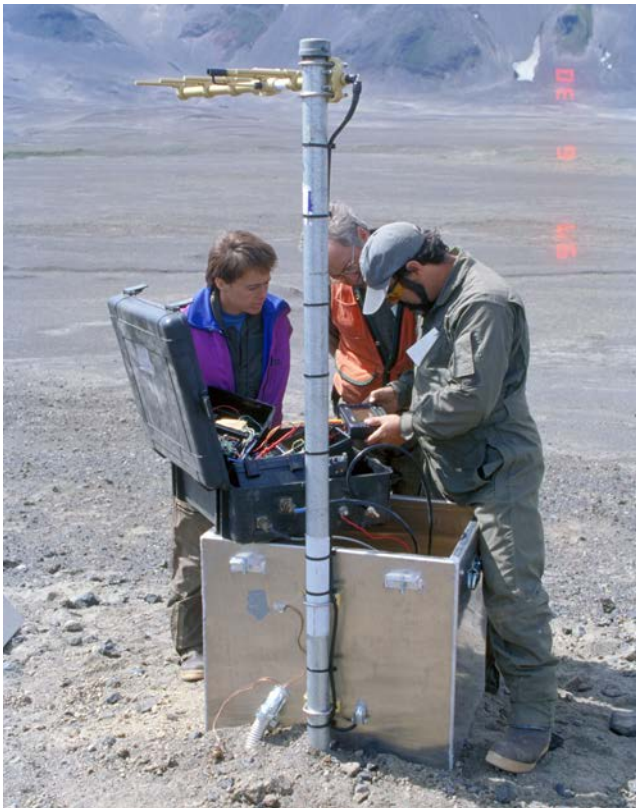
Figure 46. Photograph of AVO staff installing seismic station "Surprise Lake" (ANSL) within the Aniakchak caldera. This station is typical of the 1990s style seismic stations and was installed in 1997 and decommissioned in 2000. USGS photograph by Game McGimsey.
