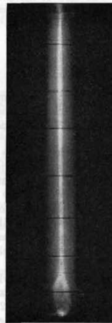
Fig. 3 The discharge showing the expanding central core surrounded by the collapsing shell during the formation on the first pinch. V = 2.5 kV; p = 500 \mu Hg.
