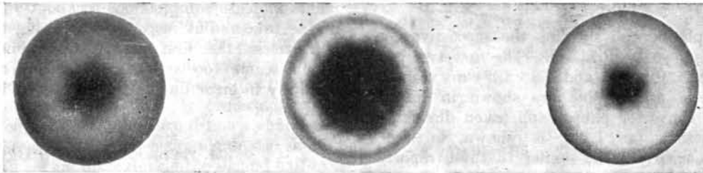
Fig. 3 Image converter photographs (exposure time 90 \text{ m}\mu\text{s} ) of an argon discharge taken at 50 \mu \text{ Hg} . Left photograph, 2.4 \mu\text{s} ; centre, 4.7 \mu\text{s} ; right, 14.8 \mu\text{s} .
