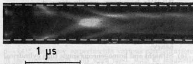
Fig. 2 Smear camera picture of preheating discharge. Initial pressure 230 \mu , D_2 .
