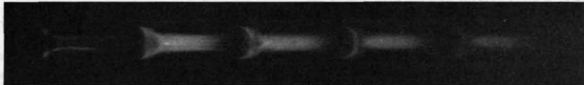
Fig. 4 Streak photograph taken in argon at 260 \mu\text{Hg} , bank voltage 18 kV, T/2 = 17.5 \mu\text{s} .
