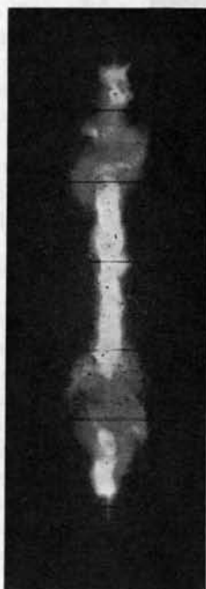
Fig. 8 Loss of containment when anode and cathode fronts approach one another. Photograph taken with conical electrodes. V = 4 kV; p = 200 \mu Hg.
