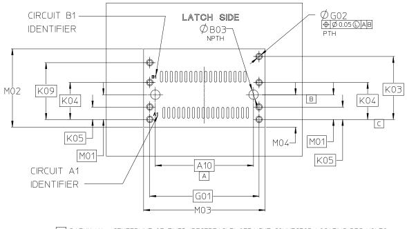
A DATUM 'A' - CENTERLINE OF FIXED (RECEPTACLE) STRAIGHT CONNECTOR LOCATING PEG HOLES
