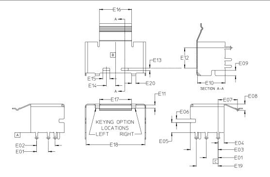
A DATUM 'A' - FIXED (RECEPTACLE) RIGHT ANGLE SHELL LOWER EDGE B DATUM 'B' - FIXED (RECEPTACLE) RIGHT ANGLE SHELL CENTERLINE C DATUM 'C' - FIXED (RECEPTACLE) RIGHT ANGLE SHELL LOCATING PEG
