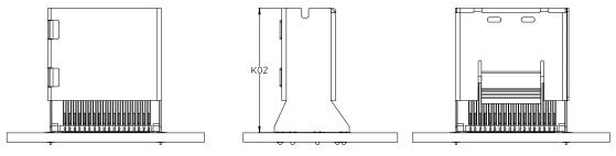
FIGURE 6-6 FIXED (RECEPTACLE) STRAIGHT CONNECTOR WITH SHELL
