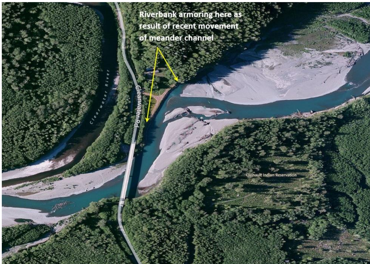
Figure 32. Queets meander channel eroding riverbank near Clearwater Road.
