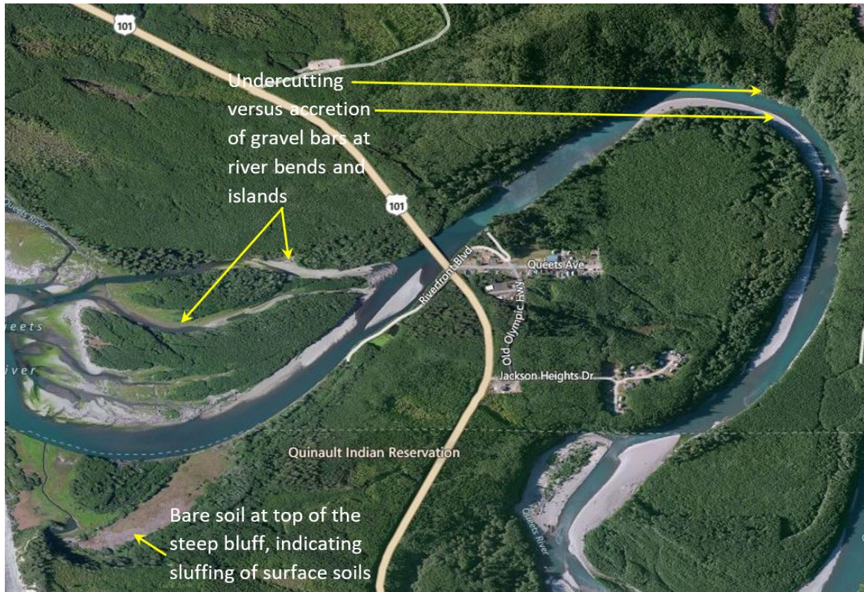
Figure 30. Erosion and slumping in glacial till substrates forming bluffs along shoreline south of the Queets.
