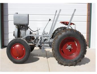
being able to operate a  $13 \ 1/2$ " plow and handle two to three acres per 10 hour day. Under maximum load, the fuel consumption was one and one half quarts per hour.
