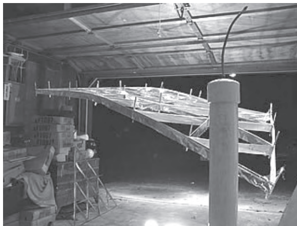
Fig. 5. Multi-Cellular Design. Multiple lifting-cells increase thrust output and overall efficiency. The Lifter-9 has 36 cells, and a combined air-gap length of 100 ft!
