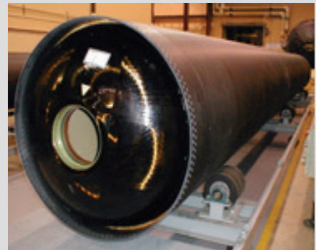
GEM cases are produced using advanced filament winding techniques developed and refined by Innovation Systems's Aerospace Structures Division for over 40 years
