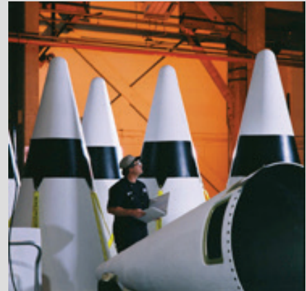
Innovation Systems's Aerospace Structures Division uses proven hand layup techniques to produce GEM 60 nose cones
