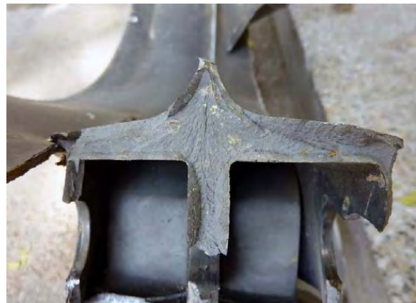
Fracture surface of LP Compressor 2 nd stage disk.
