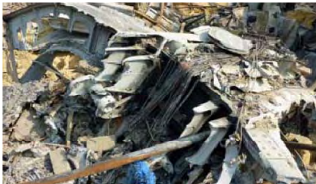
#14. Rear centre part of the stabilizer
