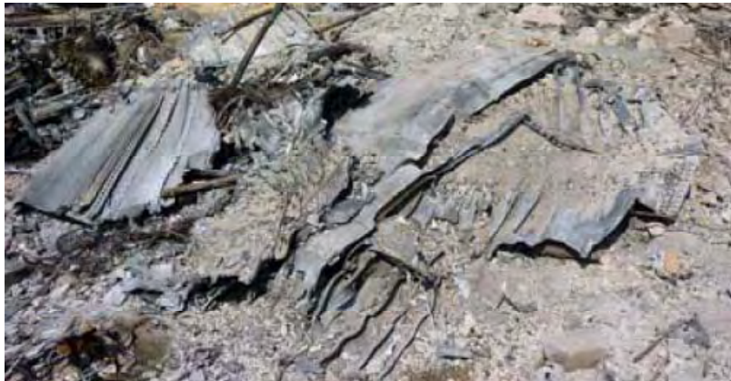
#12. Wing centre section lower panel from middle to the front spar
