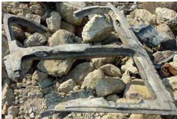
#8. Left side crew cabin transparency frame fragment
