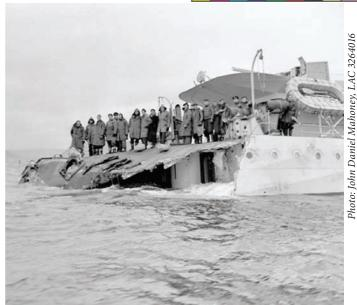
Crew stand on damaged stern of the destroyer HMCS **Saguenay**. **Saguenay**'s stern was blown off after her depth charges exploded following a collision with SS **Azra** south of Cape Race.
