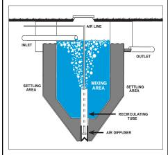
Figure 2–Another example of a possible aerobic unit design Adapted with permission from Pennsylvania State University College of Agriculture Extension Service
