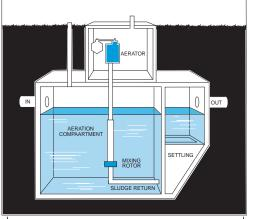
Figure 1–An example of a possible aerobic unit design Adapted with permission from Pennsylvania State
