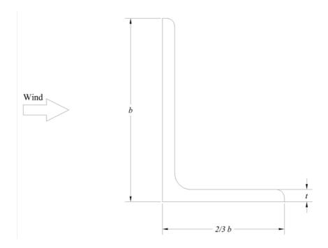
Fig. 9 L-shaped cross section. Strouhal number 0.15
