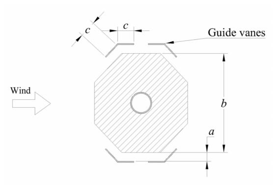
Fig. 6 Octagon cross section. c/b=0.09, a/b=0.06. Strouhal number 0.16
