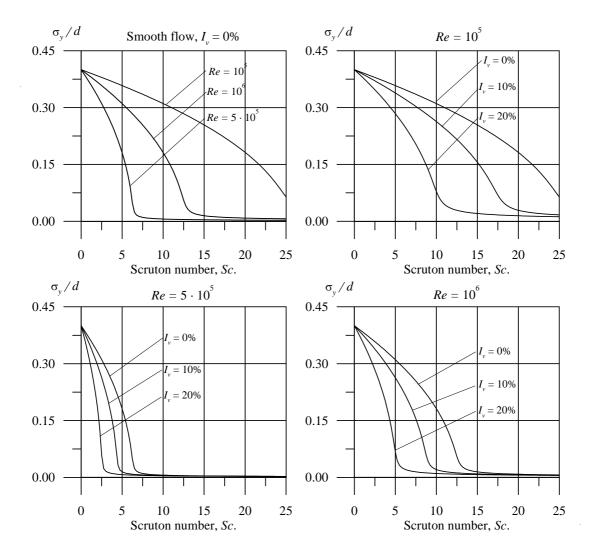
Fig. 5a-d Vortex-induced vibrations as function of turbulence intensity and Reynolds number. It is assumed that  $m_e/pd^2=50$  and h/d=30, which influence the low amplitude part of the curves shown
