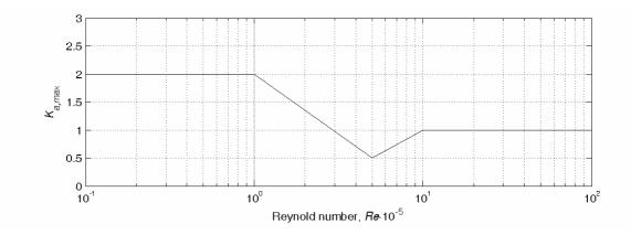
Fig. 4 Aerodynamic damping parameter  $K_{a,max}$  for smooth flow as function of Reynolds number
