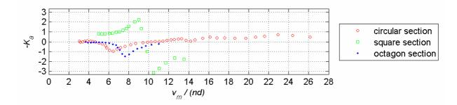
Fig. 1 Aerodynamic damping measured in turbulent shear flow for a circular cylinder, an octagon and a square. Data from Vickery (12)
