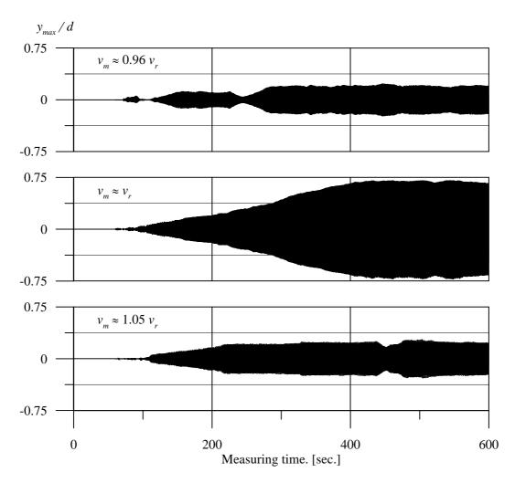
Fig. 2a-c Amplitude built-up after the cylinder has been released in low turbulence flow
