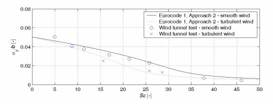
Fig. 11 Measured response and vibration predictions of L-shaped cross section based on the spectral model with  $C_{c,ref} = 0.010$ ,  $K_{a,ref} = 2.5$ ,  $a_{L,ref} = 0.050$ ,  $K_{turb} = 1.76$
