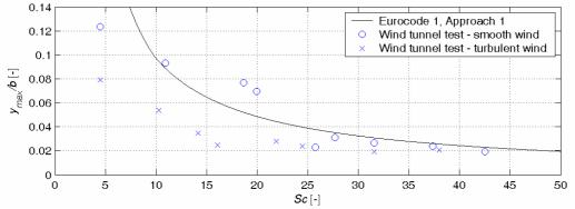
Fig. 13 Measured response and vibration predictions of bridge cross section based on the vortex-resonance model with  $K=1/(4\pi)$ ,  $K_w=0.44$  for  $y_{max}/b<0.1$ ,  $c_{lat}=0.40$
