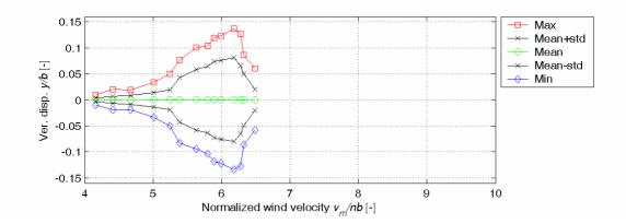
Fig. 7 Vortex-induced response of octagon cross section without guide vanes
