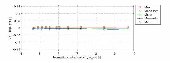
Fig. 8 Vortex-induced response of octagon cross section with guide vanes
