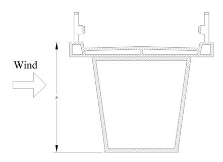
Fig. 12 Bridge cross section. Strouhal number 0.12
