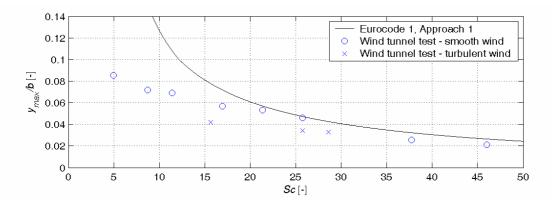
Fig. 10 Measured response and vibration predictions of L-shaped cross section based on the vortex-resonance model with  $K=1/(4\pi)$ ,  $K_w=0.53$  for  $y_{max}/b<0.1$ ,  $c_{lat}=0.65$
