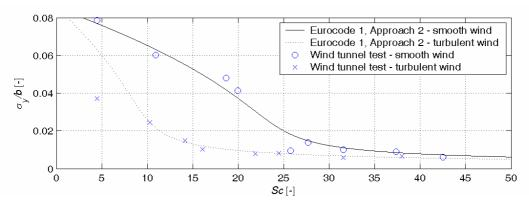
Fig. 14 Measured response and vibration predictions of bridge cross section based on the spectral model with  $C_{c,ref} = 0.009$ ,  $K_{a,ref} = 1.9$ ,  $a_{L,ref} = 0.085$ ,  $K_{turb} = 0.75$
