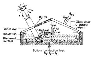
Fig. 2. Fraction of solar flux at different components of the distillation unit.
