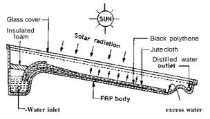
Fig. 3. Cross-sectional view of FRP multi-wick solar still.
