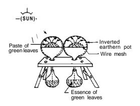
Fig. 1. Historical solar distillation apparatus.
