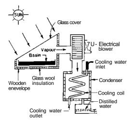
Fig. 4. Hybrid solar distillation system.
