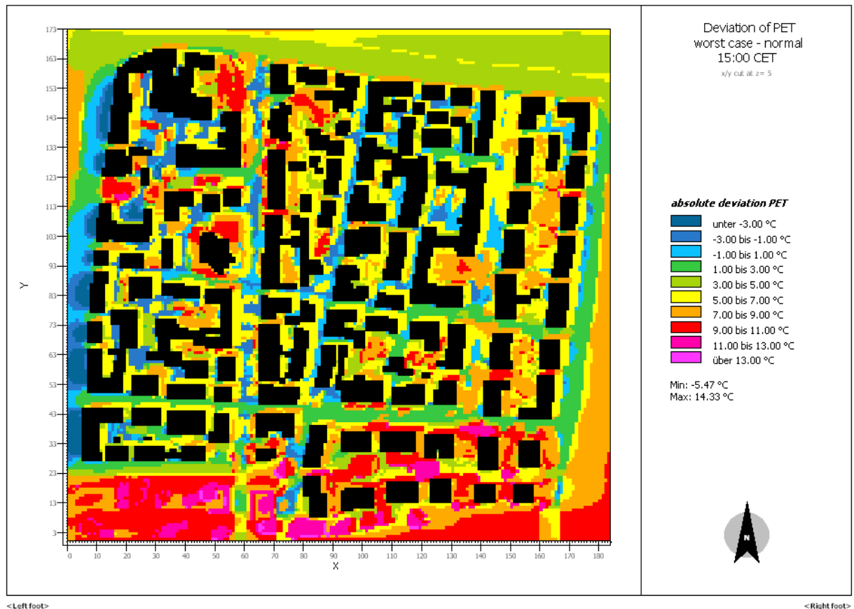
Figure 5: Comparison of PET (2m above ground) between the two scenarios (worst case - normal)
