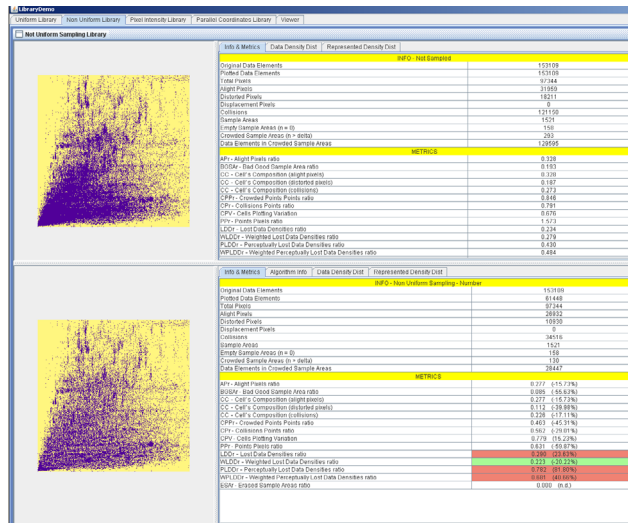
Figure 3.6: Visual data reduction preserving density differences through visual quality metrics. The image shows a curative sampling algorithm applied to the topmost scatterplot producing a more comprehensible image (below). The measurements on the right allow the user to formally assess the performance of the algorithm
