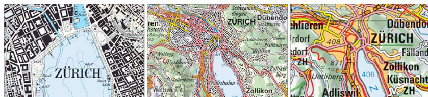
Figure 5.4: Maps show different graphical elements and different semantic content depending on the presentation's current scale. Reproduced by permission of swisstopo (BA100617) (Source: http://www.swisstopogeodata.ch/geodatenviewer/ )
