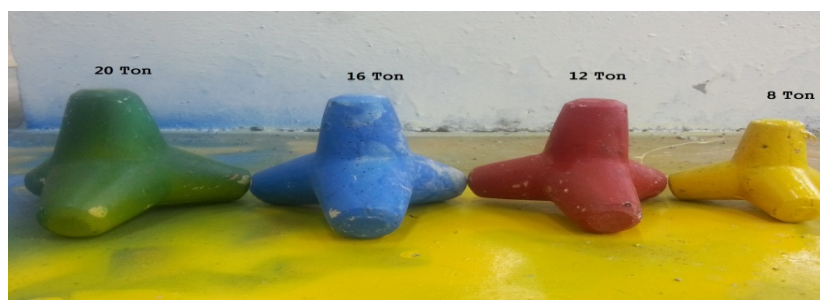
Fig. 3 Photograph of the tetrapods used in the present study.
