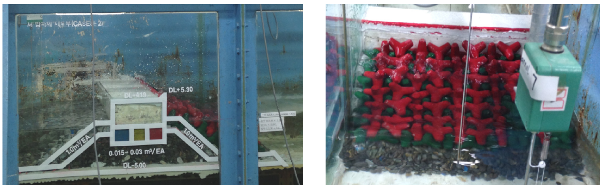
Fig. 15 Case 3 (DL+5.30), wave wall height (3.53 cm).
