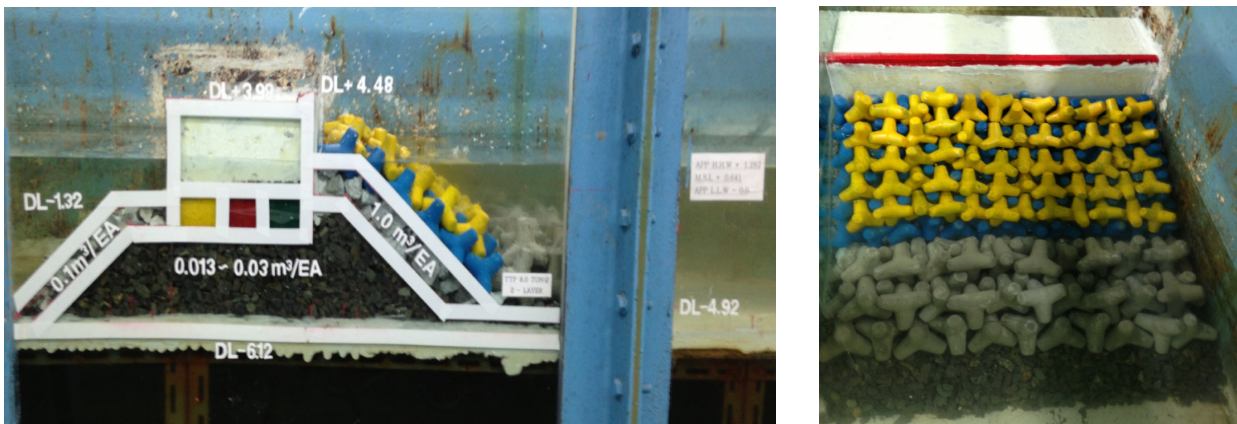
Fig. 13 Case 2 (DL+4.48), wave wall height (1.78 cm).
