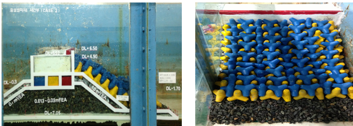
Fig. 17 Cass 4 (DL+6.50), wave wall height (6.83 cm).
