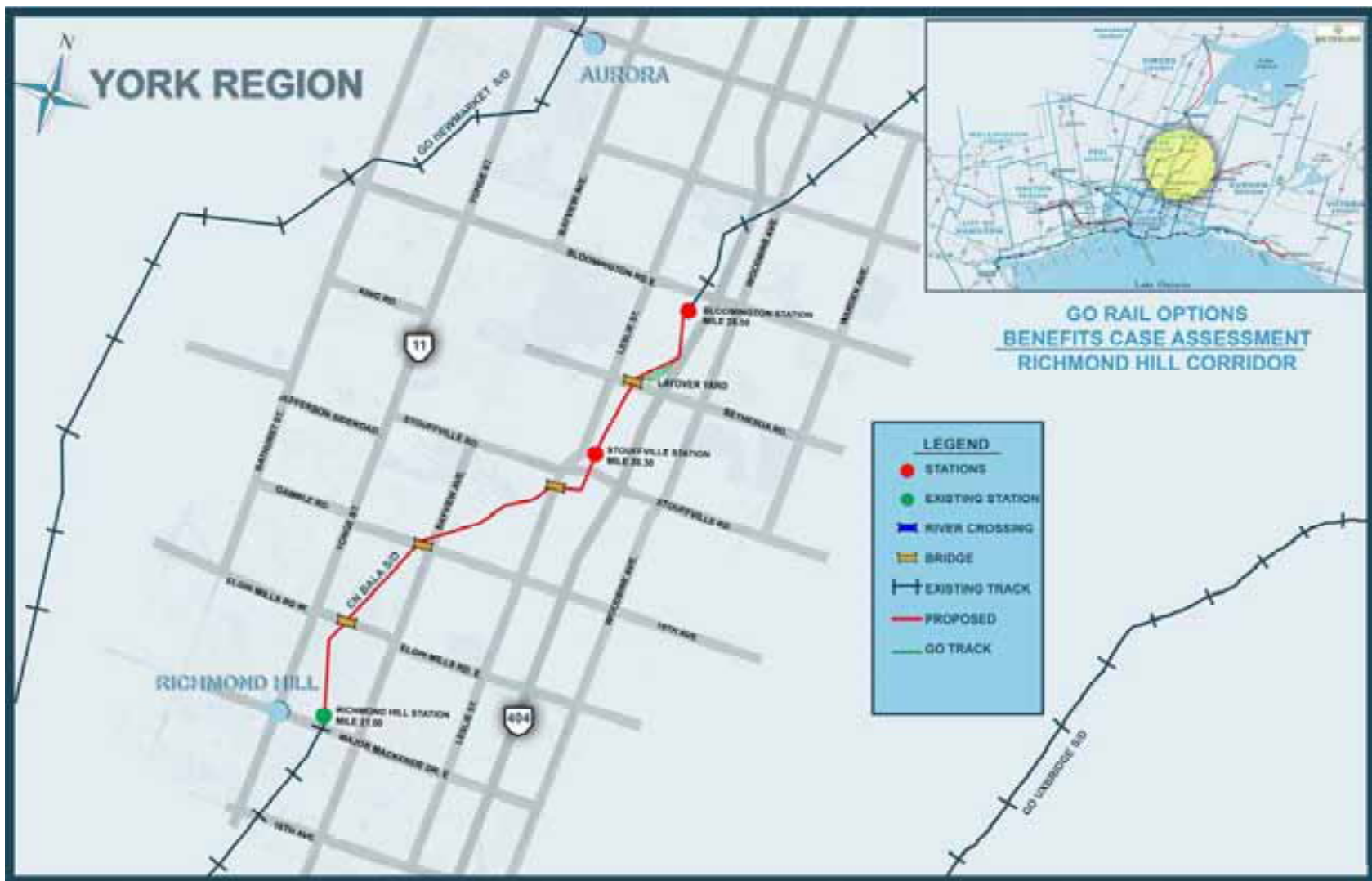
Figure 8-1: Richmond Hill (Bloomington) Proposed Alignment from Richmond Hill Station to Bloomington Station
